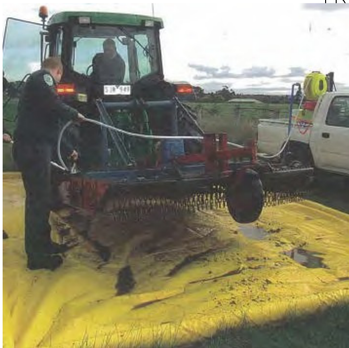
Machinery wash-down unit
