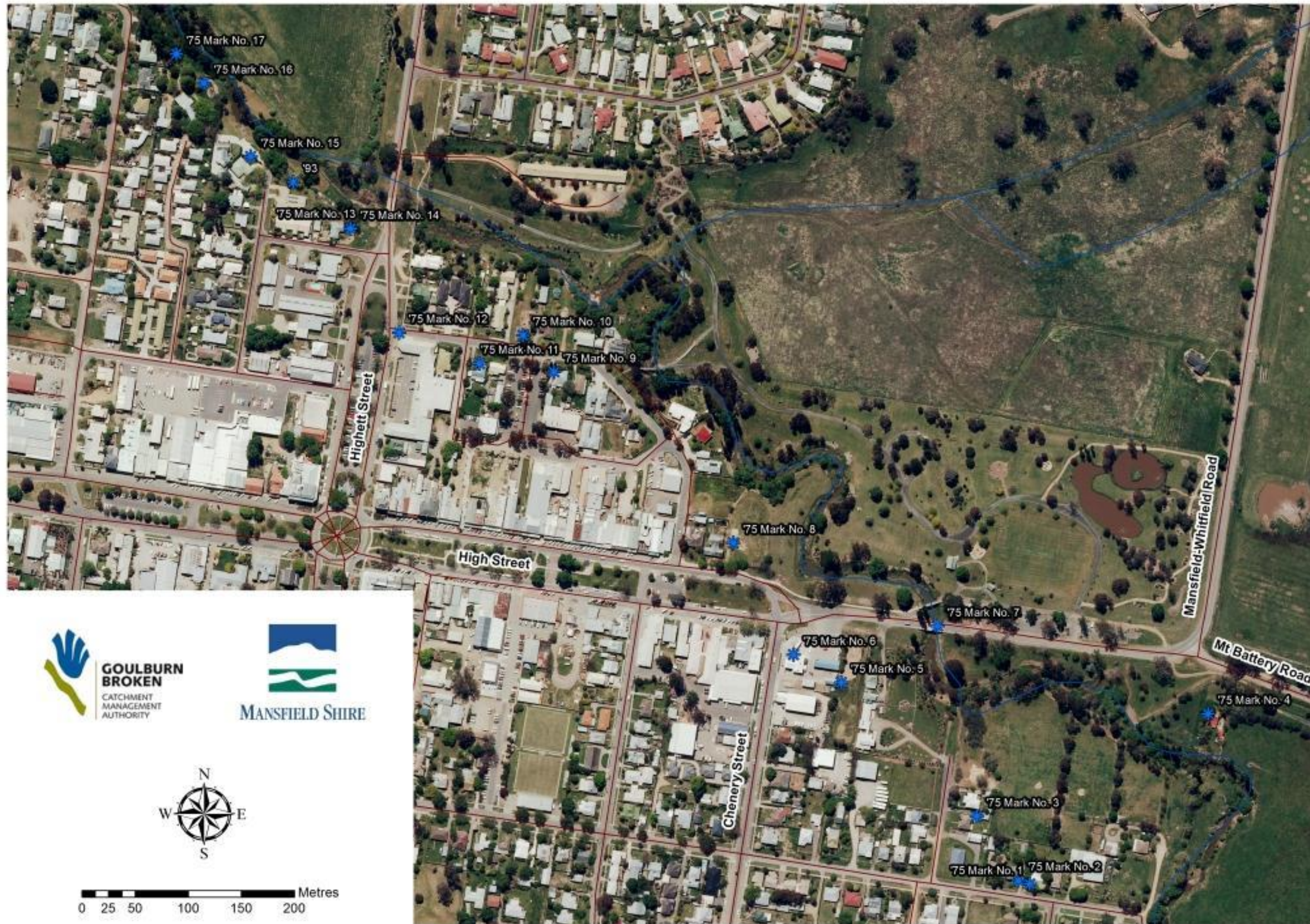
Figure 4-1 The high water marks surveyed after the 1975 flood and listed in Table 4-2.
