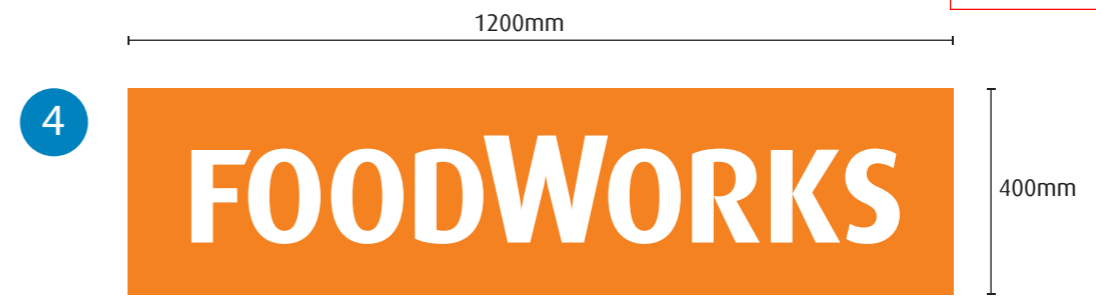
Under Awning Lightbox (Qty x1 unit - x2 faces) material LED lightbox unit; digitally printed lightbox faces location mounted below the awning as shown in mockup notes lightbox frame to be painted in FW orange
