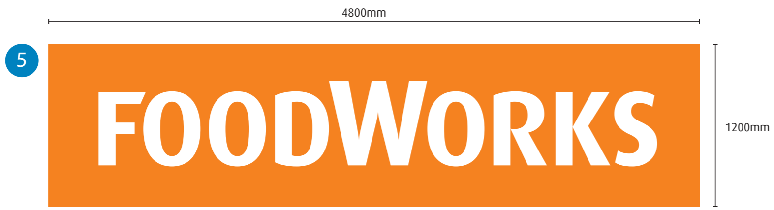
Side Wall Lightbox (x1) material LED lightbox unit; digitally printed lightbox face location mounted to the wall as shown in mockup notes lightbox frame to be painted in FW orange
