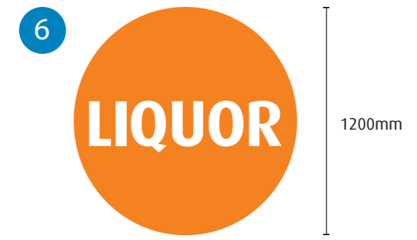
Side Wall Liquor Lightbox (x1) material LED lightbox unit; digitally printed lightbox face location mounted to the wall as shown in mockup notes lightbox frame to be painted in FW orange
