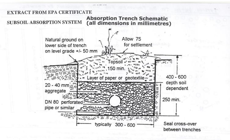
9. Subsoil absorption trenches must be sized in accordance with the following table:
